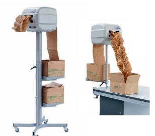
The machine is light and compact and can be handcarried. It measures 13" (L) x 13" (W) x 15" (H). Because of its small footprint it is very easy to integrate in Packing stations. The machine is easy to operate and dispenses the pads directly into the carton thus increasing productivity and Working Comfort®.
